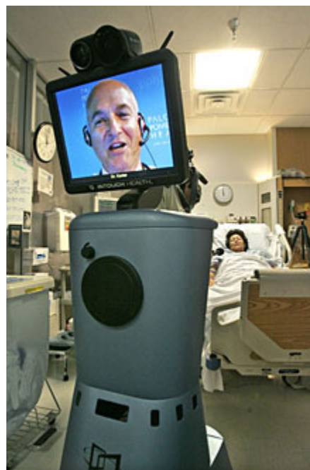
CHARLIE NEUMAN / Union-Tribune Dr. Ben Kanter of Pomerado Hospital demonstrated the RP-7 robot that is controlled by a laptop on a floor above patient Phyllis Rodriguez.
