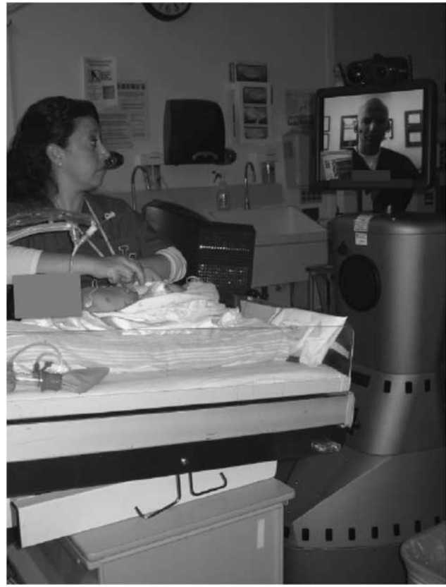
Figure 1 Telemedicine equipment (mobile robot) at patient's bedside. The robot is equipped with a pan-tilt-zoom head with a video camera, microphone, and liquid crystal display (LCD) screen and motorized platform and operates under the control of the physician at a remote site. The operator's face is projected on the screen creating a more human-type physical presence at the bedside. The operator's computer screen is also projected in the left lower corner of the screen of the robot, so that the bedside caregiver also sees what the operator of the robot is looking at on the screen of his/her station's computer at the remote site (see text for details).
